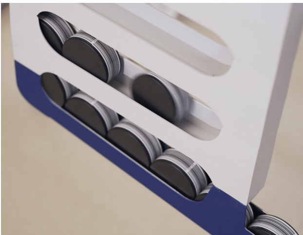
5. The sample cup is ejected into the collector after the measurement is completed. The next cup in the magazine is then loaded into the instrument.
