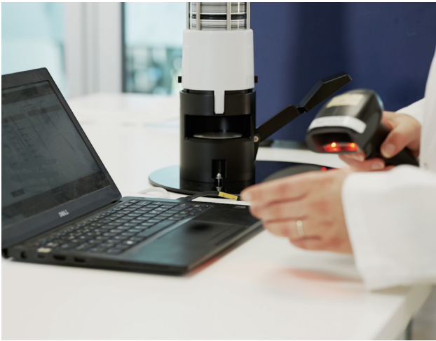
1. The sample cups are registered using the barcode on the side of the cup and then loaded into the magazine.
